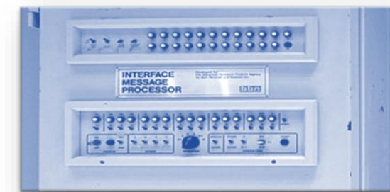
The first routers, known as Interface Message Processors or IMPs.
